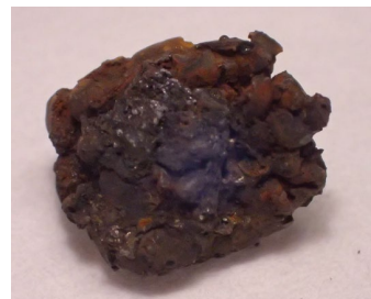
Figure 1. Appearance of the fuel debris sample [1]
