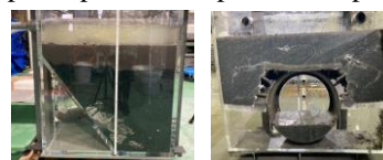
Figure 3 SIAL ® matrix with sandbag solidified under water and successful stopping leakage water
