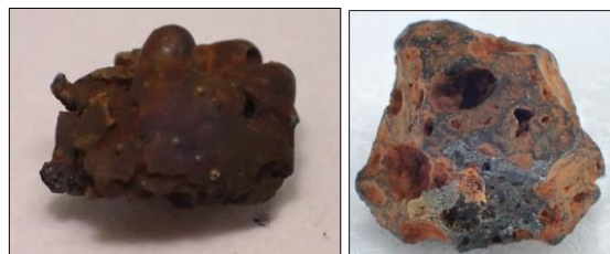
Figure 2. External appearance of Fuel Debris
