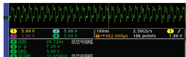
Figure 3. Ring oscillator operation.
