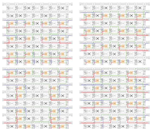
Figure 2. 4 implementation examples of a 16-bit adder circuit avoiding defects.
