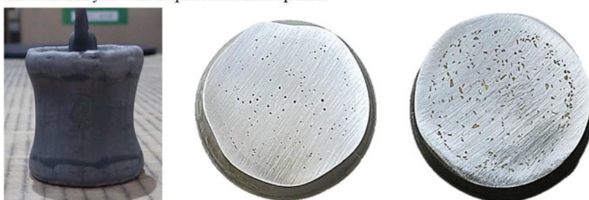
Figure 1. External appearance of HIPed waste form (left) and the cross section confining the ALPS cerium oxide (center) and silver zeolite (right) in SS matrix.
