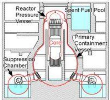
Figure 2. Cross section of P
