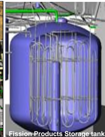
Fission Products Storage tanks
