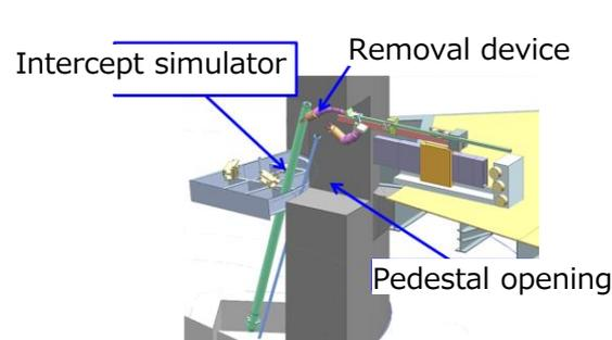
Element test of removal of interfering substance in the pedestal
