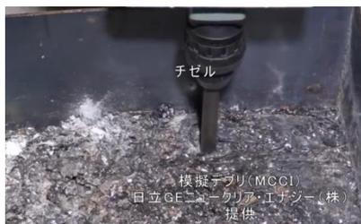
Preliminary test of chisel processing
