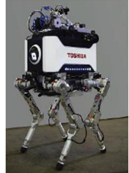
Waling survey device at the lower vent pipe
