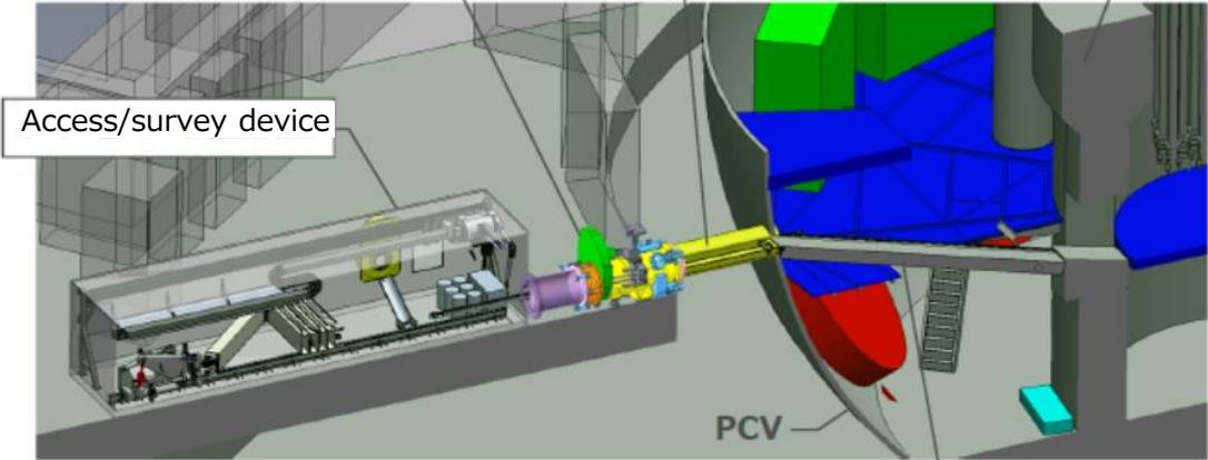
Draft plan for access/survey device installation in front of X-6
