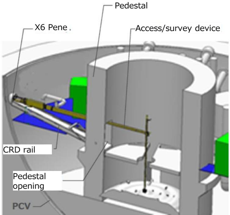
Proposed deployment of access/survey device
