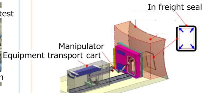
Element test of inflate seal
