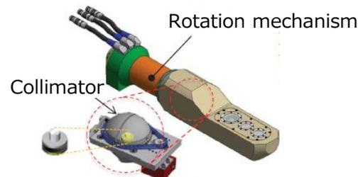
Development of radiation measurement device with gamma camera
