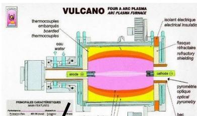
Arc Plasma furnace (For Oxide melt)
