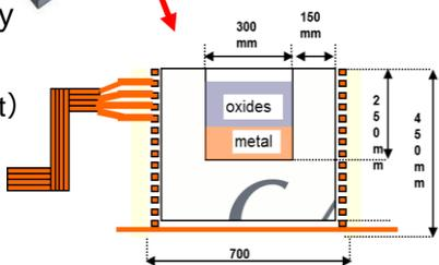
High frequency furnace (for Metallic melt)
