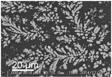
Silicate glass (containing 3-4 wt%-U) + (U, Zr, Ca) O<sub>2</sub> precipitation
