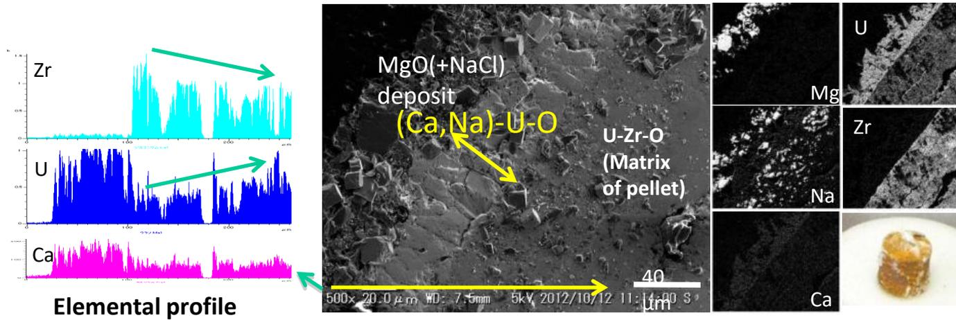
SEM images on the (U<sub>0.4</sub>Zr<sub>0.6</sub>) O<sub>2</sub> pellet Heat-treated with salt at 1275K for 12h under air flow.
