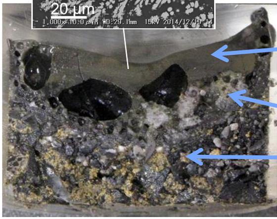
Cross section after melting reaction (Concrete piece with a diameter of 25 mm)
