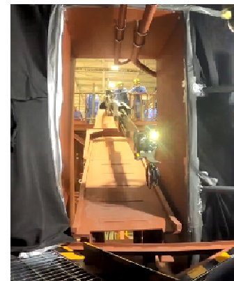
Lowering end effector from grating opening
