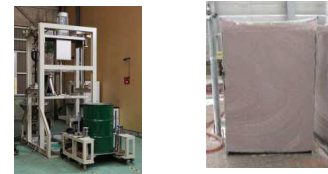
Figure 1 200L Indrum kneading machine and SIAL ® solidified body of resin
