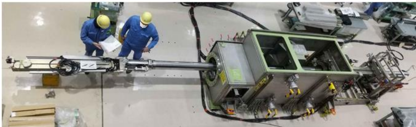
Telescopic-type device for trial retrieval (Device photographed from above)
