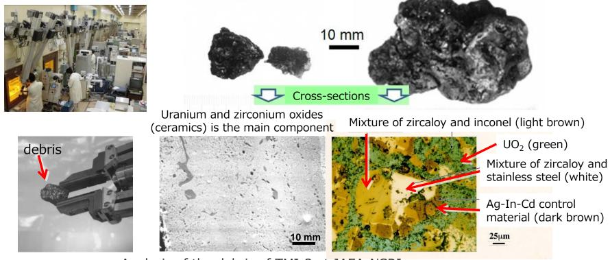
Analysis of the debris of TMI-2 at JAEA-NSRI
