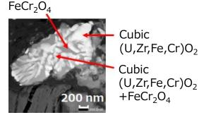
Detailed structure of U-bearing particle observed on the deposits from Unit 2 (STEM-HAADF image)
