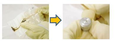
Sample preparation for SEM (Scanning electron microscope)
