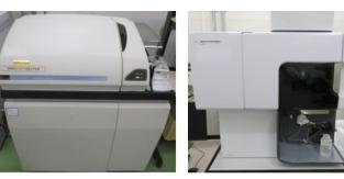
Chemical Analysis instruments (Left: ICP-MS; Right: ICP-AES)
