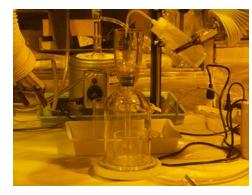
Nitric acid dissolution of simulated debris in a hot cell
