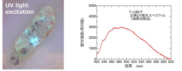
Fluorescence emitted from Type B particle irradiated with UV light
