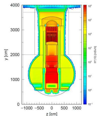
**Figure 1. Predicted Dose rate distribution in PCV of Unit-1**
