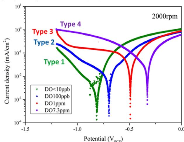
Fig.1 Results of polarization measurement
