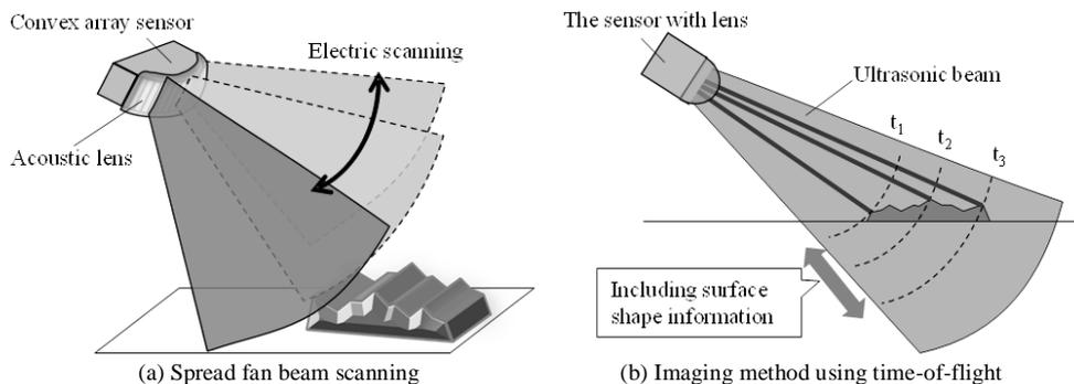
**Figure 1. Ultrasonic imaging method using convex array sensor and acoustic lens**
