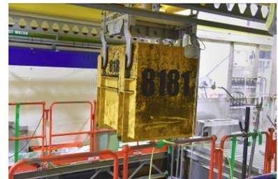
Figure 3. Metal Fuel removal from a Sellafield pond
