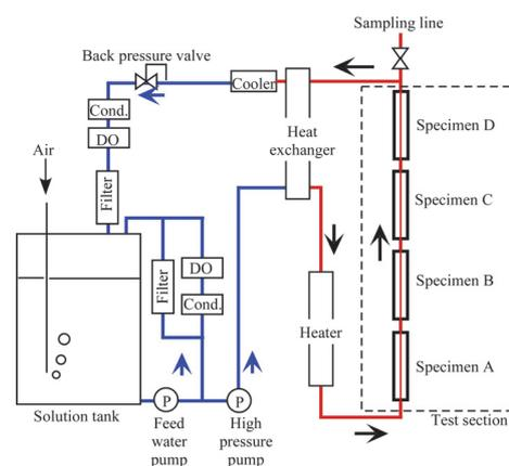
Figure 1. Schematic diagram of loop system.
