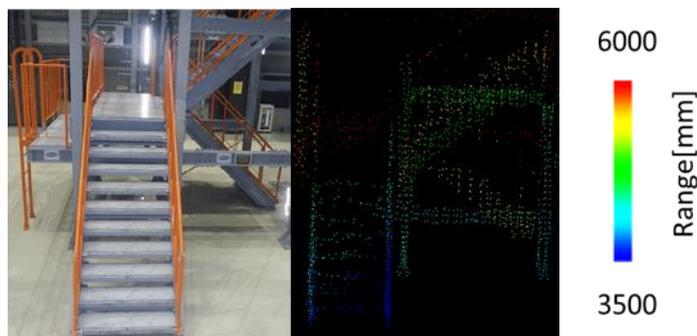
Figure 2. Laser scanner data and picture of mock-up staircase
