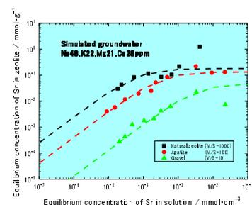
Fig.2 Absorption isotherm of Sr in simulated groundwater.
