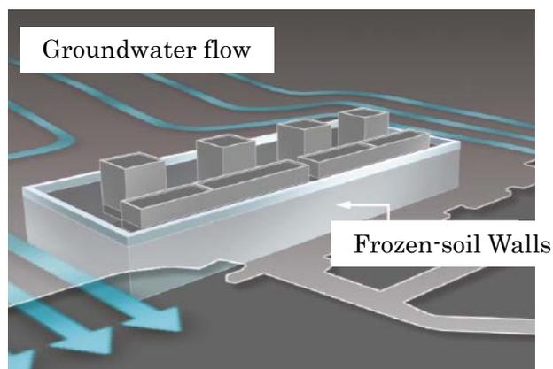
Figure 1. Concept of the Frozen-soil Walls
