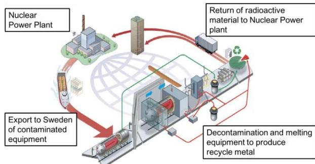
Fig. 2 Metal Recycle system flow
