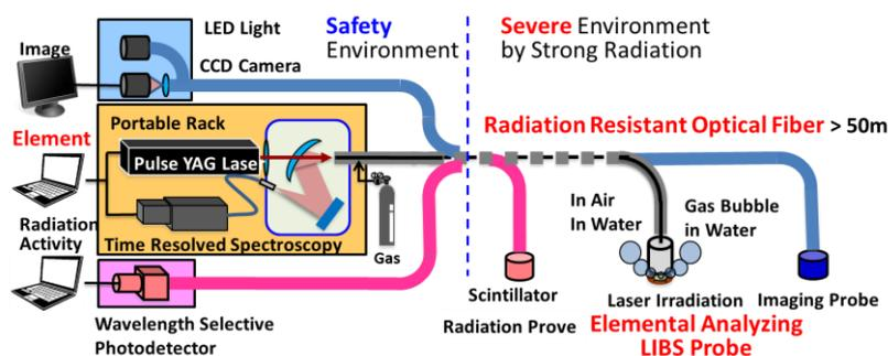
Fig.1 Concept of optical fiber based remote analysis
