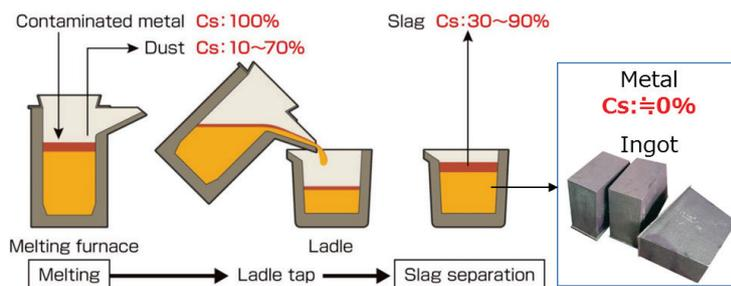
Figure 4. Process flow of radioactive Cs separation
