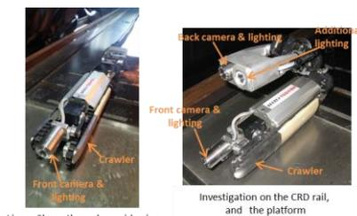
Fig.2 Investigation robot for Unit2
