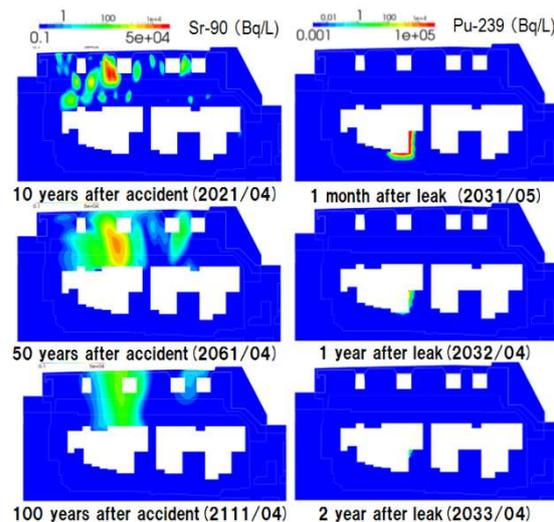
Fig.2 Behavior of radionuclides in ground water (left) reference case (right) risk case
