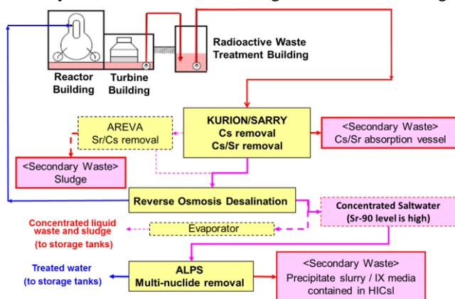
Fig.1 Overview of water treatment system
