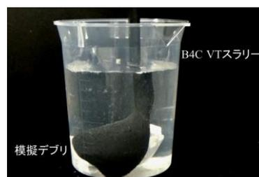
Figure1. Insoluble neutron absorbers using VISCOTOP
