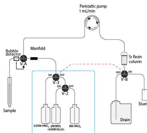
Fig. 2 Schematic layout for the automatic Sr separation system.
