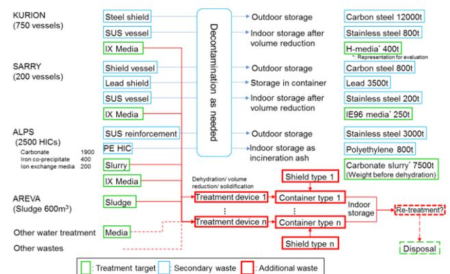
Fig.2 Quantity to be treated (quantity indicates rounded off figures for end of 2016, only major substances)
