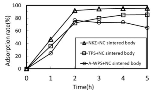
Fig1. Relation between adsorption time and Cs adsorption of porous ceramics sintered at 700°C.
