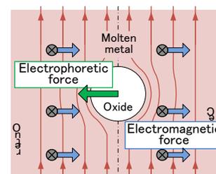
**Fig.2 Behavior of oxide in high frequency induction furnace**
