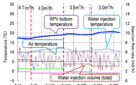
Figure 1. RPV Temperatures in Unit 2
