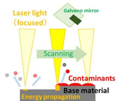
Fig. 1. Pattern diagram of laser decontamination
