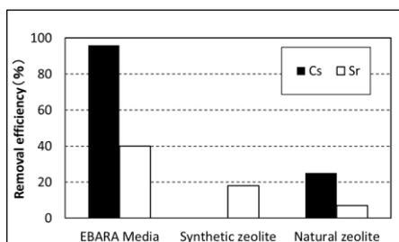
Figure 1 Cs/Sr Removal efficiency under seawater condition
