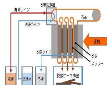
Figure2: Operational Overview (Filter Press)
