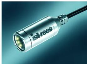
The Dotcam HR is a miniature color camera designed for use in higher radiation environments, up to a total absorbed dose of 100krad (1kGy), and being equipped with an integral white LED lighting ring, 4.0mm f/5.0 lens and is fully immersible to a depth of 60m.
