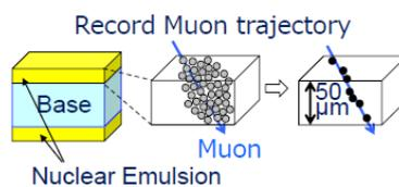
Fig.1 principle of muon detection
