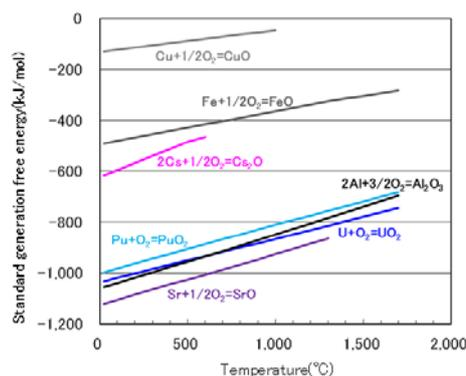
**Fig.1 Oxide formation free energy of main metals**
