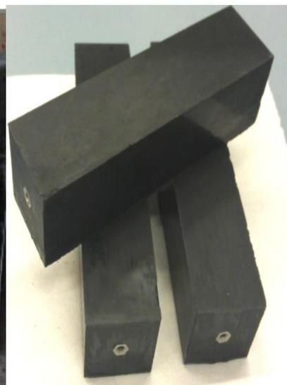
Figure 2 : Oil/ geopolymer composite
