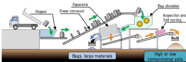
Figure: Conceptual Design of ISF Process Train
