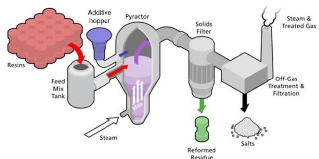
Fig. 1 THOR treatment process flow
