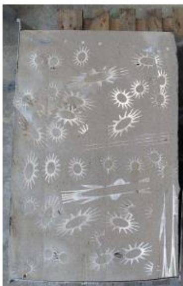
Figure 1: Encapsulation of Mg cladding in geopolymer
