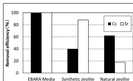
Figure 2 Cs/Sr Removal efficiency under diluted seawater condition
