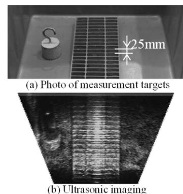
**Figure 2. Measurement results of our proposed imaging method**
