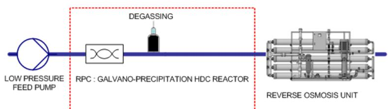
Figure 1 P&ID of typical system
