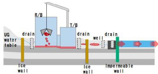
Fig. 1 Assumed pathway of contaminated water
