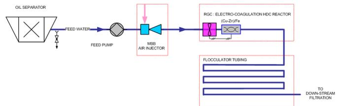
Figure 1; P&ID of typical system
